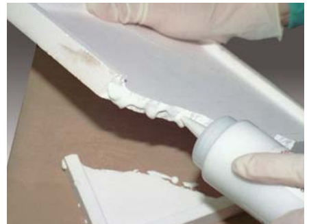
Cerabond™ 503 repairs furnace saggar plate.
