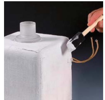
Ceramabond™ 569 bonds flex heater to quartz vessel.
