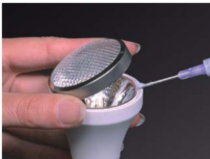
Cerabond™ 835-M bonds cover to halogen lamp.
