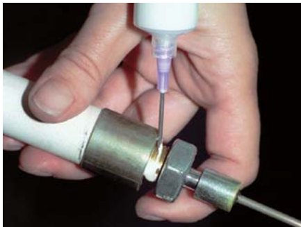
Cerabond™ 671 used as a high temp threadlocker.
